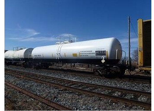
A tank car designed for transporting hydrogen peroxide by rail
