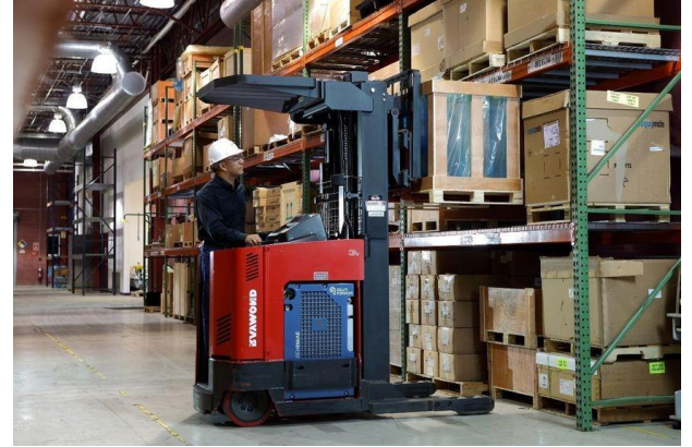
A reach truck powered by Plug Power; Amazon is a big Plug Power customer. Image courtesy Plug Power
